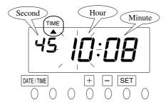
1 Push the DATE/TIME button for 1 second and position the "▲" under the "TIME" mark.
