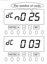
Push the reset switch with a pointed implement while pushing the FUNCTION and button. Then, the number of cards that you are using will be shown on display.
