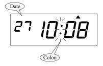
Push the <u>SETTING END</u> button to get out of the setting mode.
