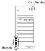
When you select "1: V/VN Card", the clock will remember the last imprint and automatically switch the "IN" and "OUT" columns by distinguishing each card with barcode. (Up to 100 cards can be used for one period.)
